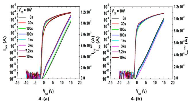
**Figure 4.** Variation in the  $I_{DG}$ – $V_{GS}$  transfer characteristics for the (a) ITO and (b) Ti devices as a function of the stressed time for  $10^4$  s under a drain-bias stress of 20 V.  $V_{DS}$  of 10 V was applied for the measurements. Negative shifts in  $V_{TH}$  for the ITO and Ti devices were estimated as 2.06 and 0.96 V after the positive drain-bias stress, respectively.
